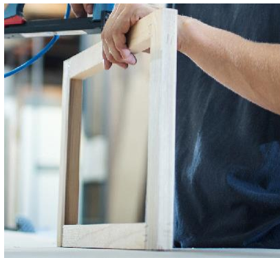
Butt-joint glued and stapled
